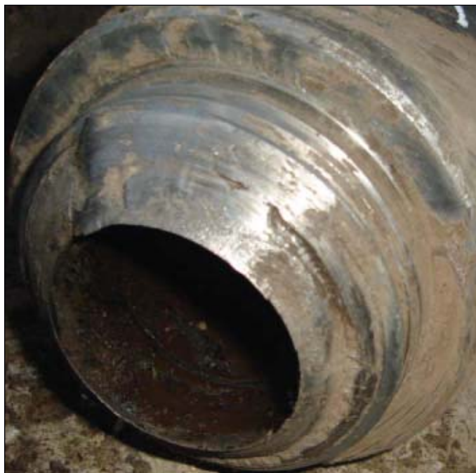
In Well Milan 1 (photo on the left), the fracture failure in a 120.7 mm (4¾ in.) drill collar is in the pin's last engaged thread (Fig. 3). During January-March 2006, six 158.8 mm (6¼ in.) drill collars broke at the box (photo on the right). The fractures were 102-110 mm from the box seal shoulder, as seen in this failure from Well Gucheng 4 (Fig. 4).
