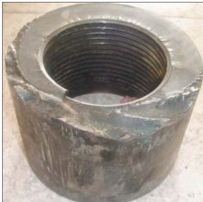
In Well Milan 1 (photo on the left), the fracture failure in a 120.7 mm (4¾ in.) drill collar is in the pin's last engaged thread (Fig. 3). During January-March 2006, six 158.8 mm (6¼ in.) drill collars broke at the box (photo on the right). The fractures were 102-110 mm from the box seal shoulder, as seen in this failure from Well Gucheng 4 (Fig. 4).
